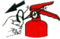
Pull the plastic tab off the fire extinguisher handle
